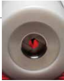
The Iris Collimator includes two banks of six tungsten segments capable of rapidly manipulating beam geometry to deliver up to 12 unique beam diameters from each linac position.
