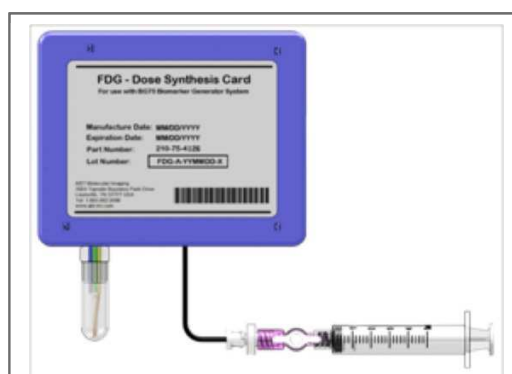
Figure 4. ABT Biomarker Generator Dose Synthesis Card (DSC) for generating a single dose of ^{18}F FDG radiopharmaceutical. This ABT consumable consolidates multiple, separate subcomponents of conventional radiochemistry systems into a single disposable item.
